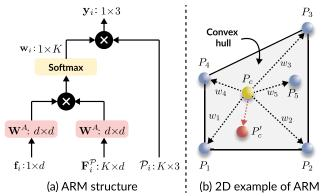
Figure 3. A 2D example and details of our proposed ARM, which re-samples a point  $P_c$  to  $P'_c$  from the convex hull by adjusting the weights  $w_i$ , i = 1..5.
