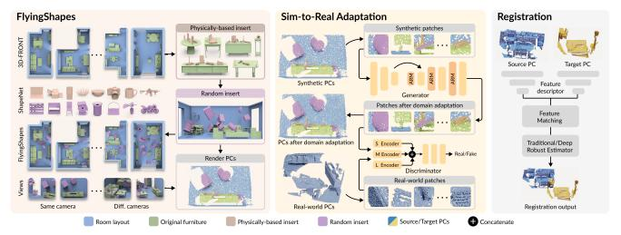
Figure 2. Our SIRA-PCR framework: (i) FlyingShapes is a large-scale indoor synthetic dataset for point cloud registration, which is constructed by applying physically-based and random strategies to insert ShapeNet models into the 3D-FRONT scenes; (ii) SIRA is then applied for sim-to-real domain adaptation on point cloud patches; (iii) the generated synthetic dataset is used to train registration models.
