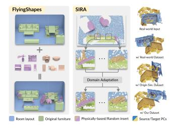
Figure 1. We construct the first large-scale scene-level synthetic dataset for point cloud registration, called FlyingShapes, by inserting objects into simple indoor scenes through physically-based and random strategies. Then, a generative-based pipeline, named SIRA, is designed for sim-to-real adaptation. Qualitative results show the performance improvement of our approach.
